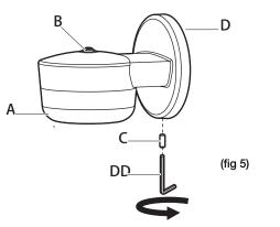
10. Apply a small bead of silicone (not included) per manufacturer's instruction around the perimeter of the fixture (A) where it contacts with the surface of the wall or ceiling.
